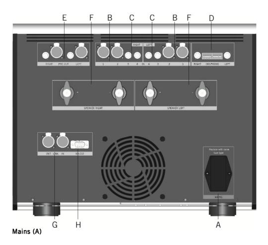
Connect the integrated amplifier 530 with the mains. After switch-on, the 530 changes to operating condition OFF (red LEDs in display, consumption <0.5W).
