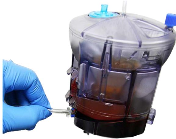
*Figure 4: Buffy Coat Sample Access Tube identified and squeezed*
