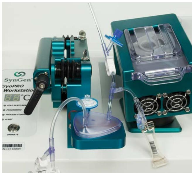
*Figure 7: Mixing Chamber in Rotating Mixing Chamber Holder with DMSO Filter at 12 o'clock*
