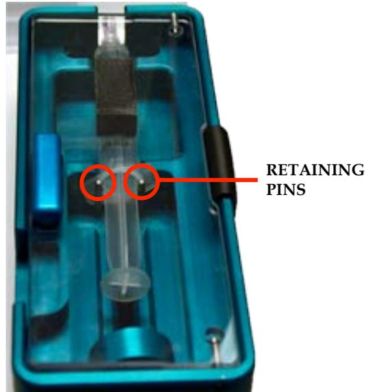
*Figure 13: Flanges of syringe above retaining pins*
