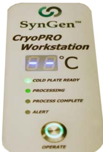
*Figure 11: COLD PLATE READY light illuminated*
