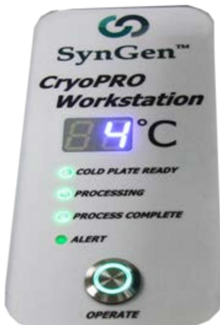
*Figure 15: PROCESS COMPLETE light illuminated*
