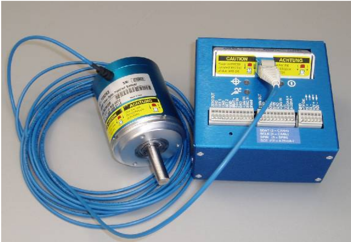
Figure 1 Micronor MR330 Fiber Optic Position Sensor System
