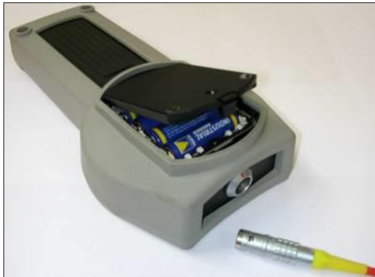
Battery compartment & flylead socket
