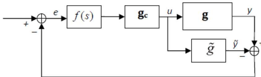
Figure 2.11: The internal model control (IMC) structure
