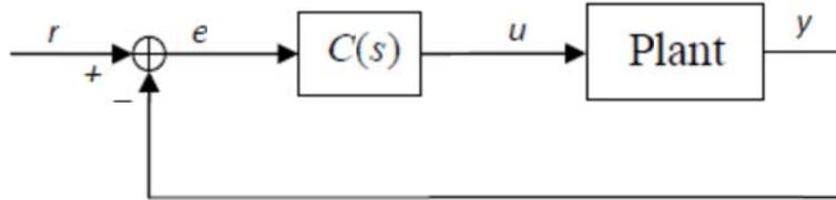
Figure 2.12: Closed-loop system with IMC controller (Jahanshahi and Skogestad 2013)
