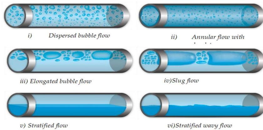
Figure 2.1: Gas-liquid flow regimes in horizontal pipes.
