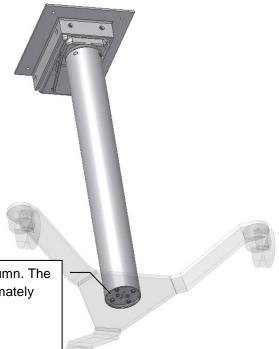
Use all four screw holes to fit the foot to the column. The screws should be long enough to enter approximately 20 mm into the column. Tighten the bolts with a maximum torque of 10 Nm.
