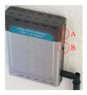
You might have to plug in the socket from the power suply (A) as it might be hooked up to the lower broadband router and even change the cables from the "broadband feeding" cable (B) to the upper box if the cabled version of internet was used previously.
