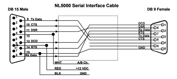
The above interface cable facilitates the connection of standard RS-232 signals to a typical 9 pin "D" type female connector. This cable additionally accommodates the connection of the +12 VDC, Ground and the A/B power or channel selector to the 15 pin "D" type female connector on the NL5000 front panel. As shown, D1 is placed in series between pin 6 and the + 12 VDC supply voltage and provides reverse polarity protection.
