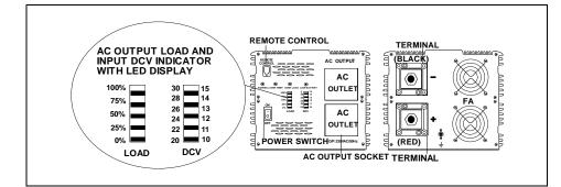
CAUTION : DO NOT REVERSE INPUT. USE RED BATTERY CORD TO CONNECT (+) OF A DC BATTERY TO (+) TERMINAL. AND THEN, USE BLACK BATTERY CORD TO CONNECT (-) BATTERY TO (-) TERMINAL.
