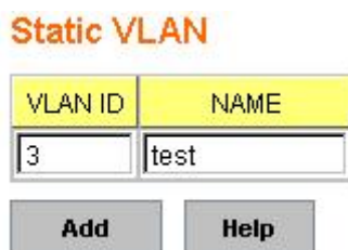
Figure 4.6.2.2 The steps to create a new VLAN: Type VLAN ID and NAME, and press Add to create a new VLAN. Then you can see the new VLAN in the Static VLAN Configuration table. Refer to Figure 4.6.2.3
