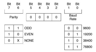
If bits 2, 3, 4, 5 are not zero, the MOF will default to the following parameters: 9600 bauds, ODD Parity, Slave Address of 1.
