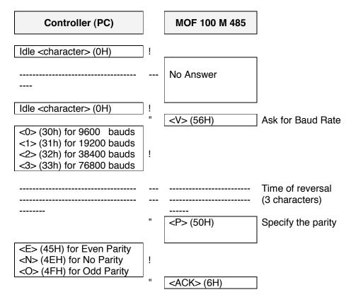
The new configuration will be valid only after cycling power to the unit. Until then, the speed of communication remains in 4800 bauds.
