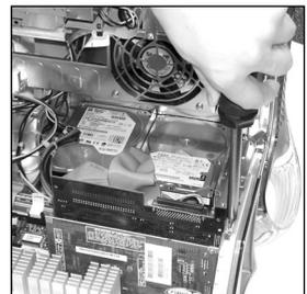
4. Insert the card carefully, and make sure that it is fitted properly into the slot.
