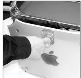
3. Remove the screw and the blind panel on the PCI slot you are planning to use.
