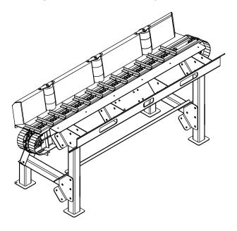
The logs are laid on the longitudinal conveyor and fed hydraulically into the machine.
