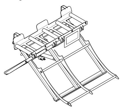
The log can easily be raised with the hydraulic lifting device.
