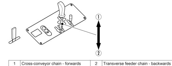
Using the control lever (cross-conveyor chain - forwards) move the log up to the longitudinal or roller conveyor.
