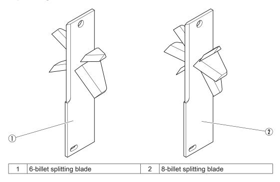
The log is split into 4, 6 or 8 pieces (billets) in one splitting process.
