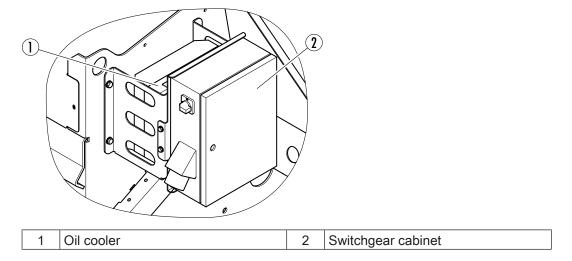
The oil cooler protects the hydraulic system against high temperatures and hence the need for frequent maintenance.
