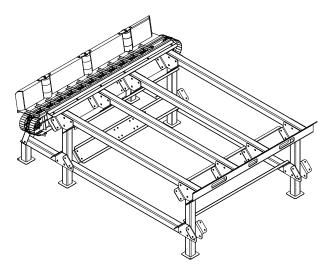
The logs are laid on the cross conveyor and fed hydraulically to the longitudinal or roller conveyor.
