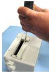
Figure 31: Opening Secondary Cable Slot
