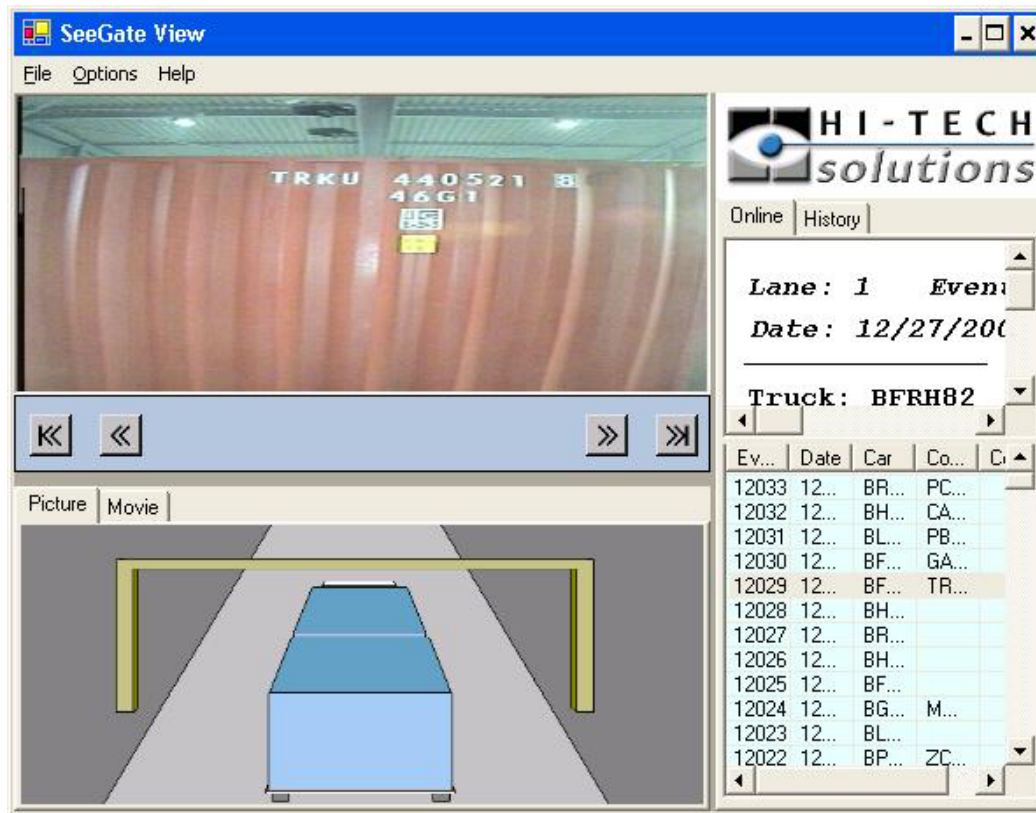
Photo 4.5: SeeGate view: A viewer for the on-line and past events
