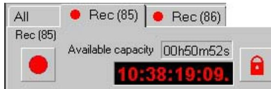
The recorder is represented by a Record button and the Record time, the duration already recorded and a lock/unlock record button. To start and to stop the record, press the Record button. If no TimeCode reference is entered to the XT Series Server, then the internal PC clock of the XT Series Server is used as a reference.
