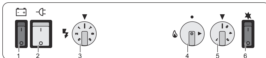
Fig. 90 Operating controls for refrigerator (electric ignition)
