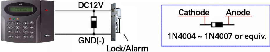
Figure: Reverse Diode Connection
