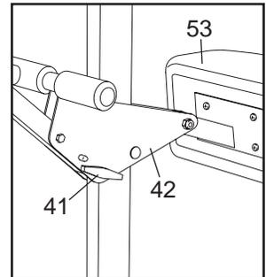
Tighten the Adjustment Knobs (41) to hold the Hip Pad (53) in position. Make sure both Knobs are secure.
