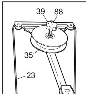
Note: As you turn the Resistance Knob to increase the resistance, the numbered Resistance Scale Decal (88) will protrude through the Knob to show the resistance settings.
