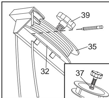
Fully loosen but do not remove the Resistance Knob (39). Lift the Pulley (35) and roughen the surface of the leather Resistance Pad (32) with 100-grit sandpaper or a file.
