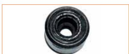
interior ring damaged for 100%
