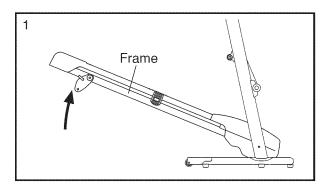
Hold the treadmill firmly with your right hand as shown. Pull the latch knob to the left and hold it. Raise the frame until the catch is past the latch pin. Then, slowly release the latch knob; make sure that the catch is resting against the latch pin.
