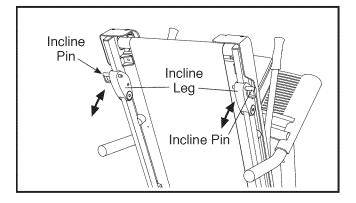
To change the incline, first remove the incline pin from one of the incline legs. Adjust the incline leg to the desired position, and then fully reinsert the incline pin. Adjust the other incline leg in the same way. **CAUTION: Before using the treadmill, make sure** that both incline legs are at the same height and that both incline pins are fully inserted into the incline legs.
