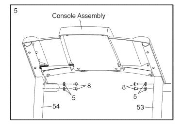
Start an M8 x 15mm Bolt (8) with an M8 Star Washer (5) into each Upright (53, 54). Then, firmly tighten all six M8 x 15mm Bolts (8).
