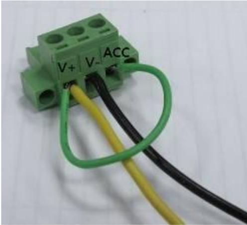
2. Power On with ACC control: ACC connector to ignition switch.
