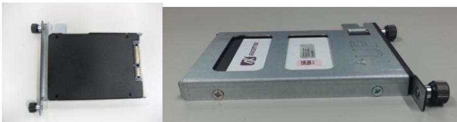
**Step 3** Slide CFast card or HDD/SSD into slot carefully
