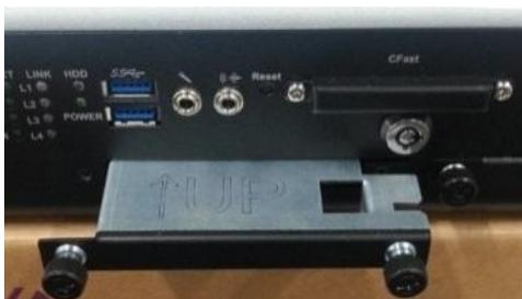
**Step 2** Assembly the HDD/SSD bracket together with the SATA HDD/SSD
