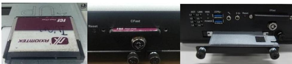
**Step 4** Fasten screws of HDD/CFast bracket
