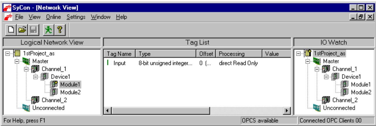
Figure 53: Logical Network View and I/O Watch
