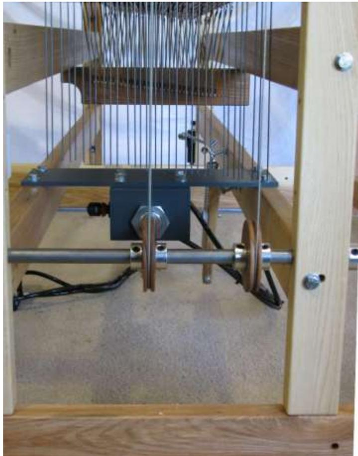
**FIGURE AL-3: Cable Routing (Right Side of Loom)**
