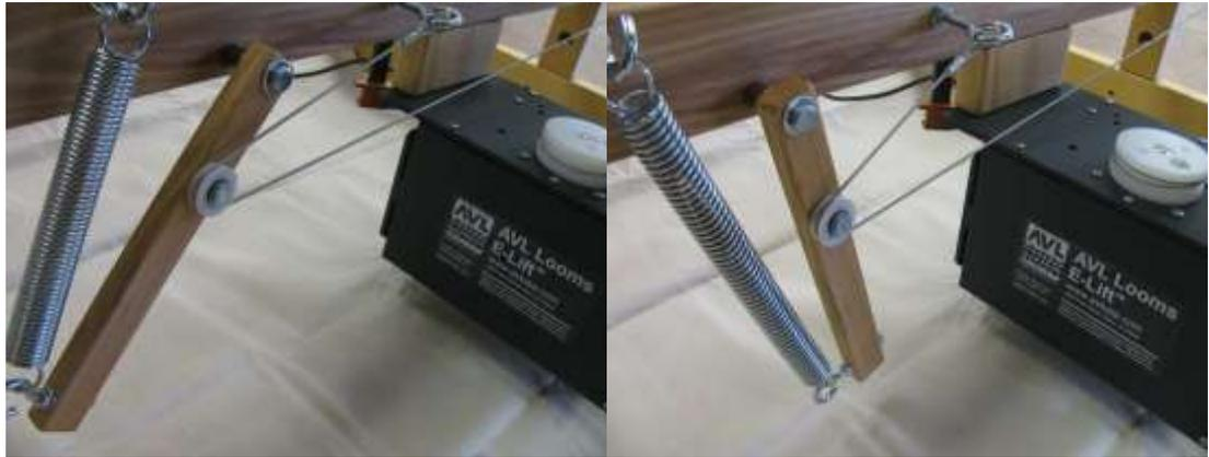
Figure EL-7: Spring Lever Position at Slide Plate Up (Left) & at Down (Right)
