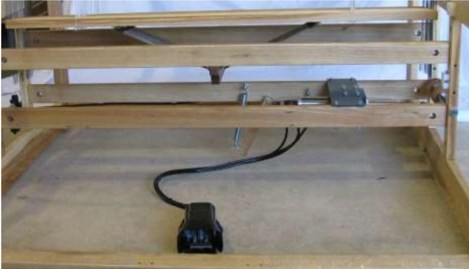
FIGURE AL-1: A-Lift on A-Series Loom (front)
