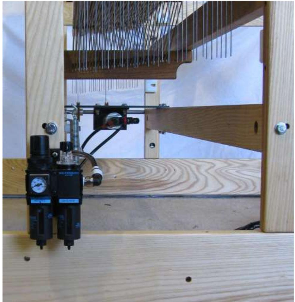
**FIGURE AL-2: FRL Placement (Left Side of Loom)**
