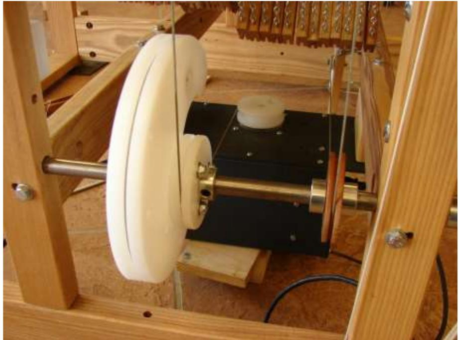
**FIG. 8-B: E-Lift Dobby Cam-Cylinder & Pulley**
