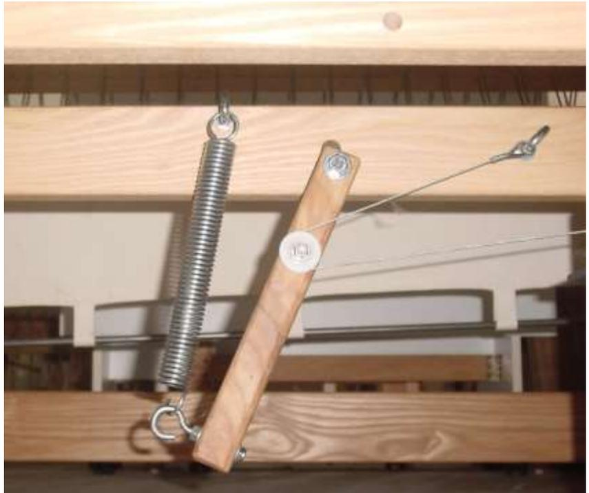
FIGURE AL-4: Spring Lever with Cable Routing
