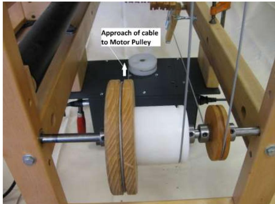
**FIGURE EL-6: Path of Motor-To-Cam Cable**
