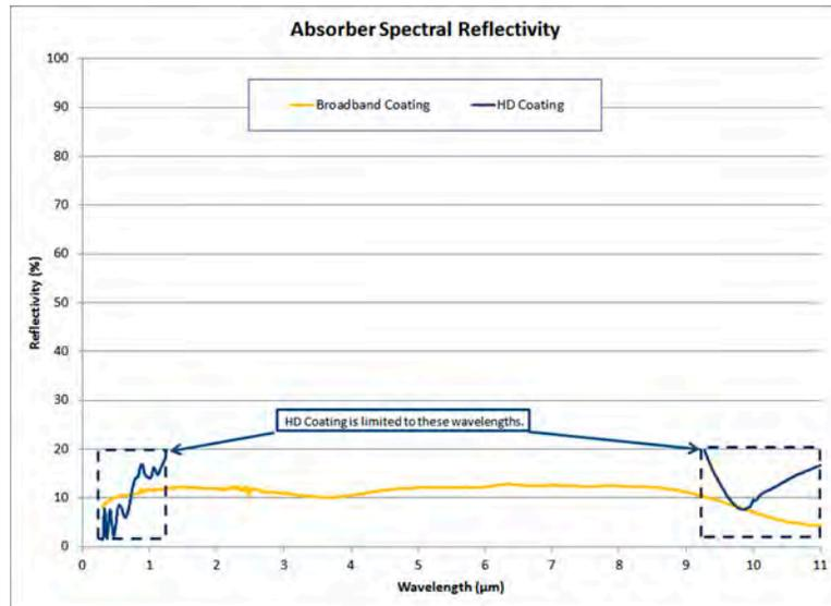
**Figure 2-7. RV Spectral Correction for PowerMax-Pro Sensors (Normalized to Calibration Wavelength)**
