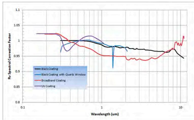
**Figure 2-6. RV Spectral Correction for Thermal Sensors (Normalized to Calibration Wavelength)**
