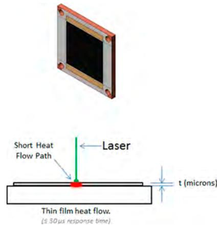
**Figure 2-4. Basic Configuration of a PowerMax-Pro Sensor**
