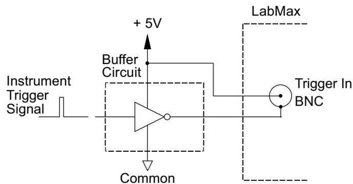
**Figure 3-5. Boosting Source Current of Triggering Device**
