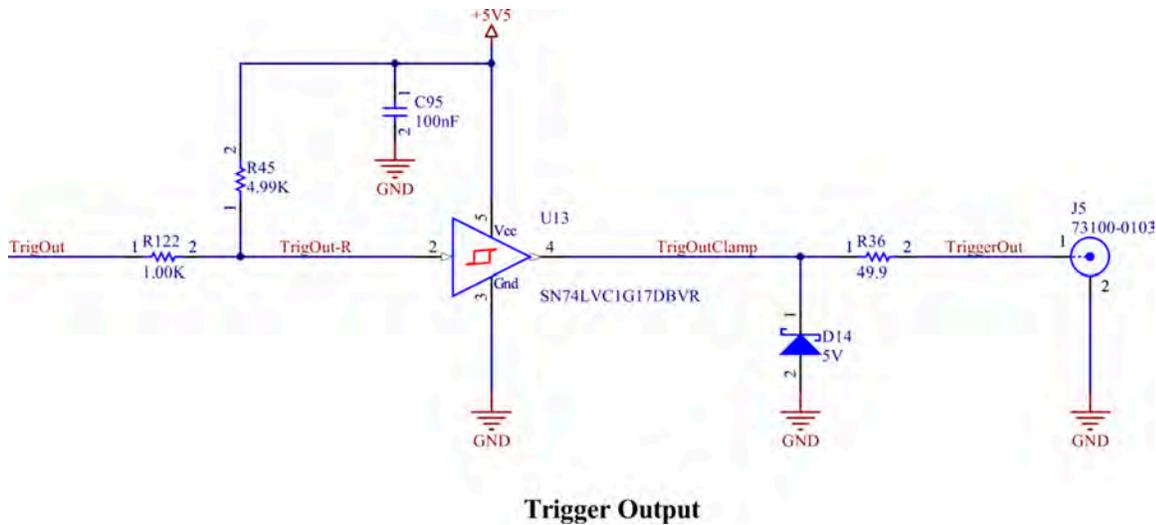
Figure 3-6. External Trigger Output Circuitry
