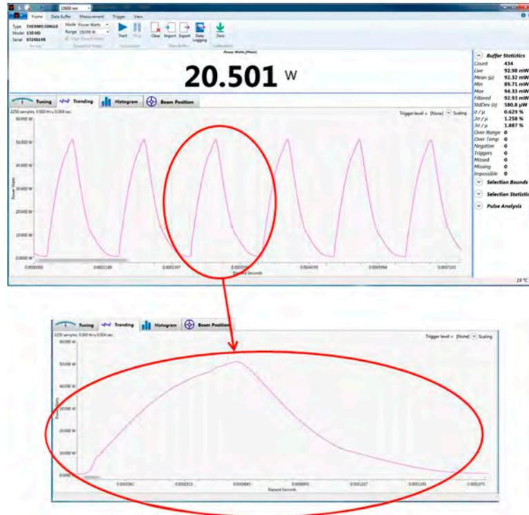
Figure 2-2. Example of Detail Available When Using Snapshot Mode
