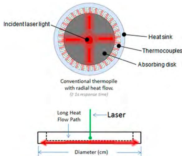
Figure 2-3. Construction of a Traditional Radial Thermopile
