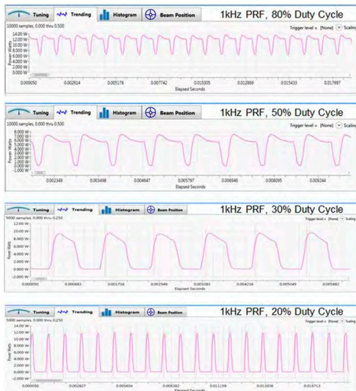
Figure 2-1. Example of Detail Available When Using High-Speed Mode
