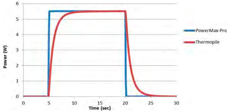
**Figure 2-5. The Rise Time of a Typical Mid-power Thermopile (30W) Compared with the PowerMax-Pro**
