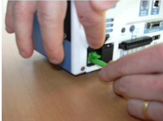
Figure 4 Connection of the fiber optics lead
