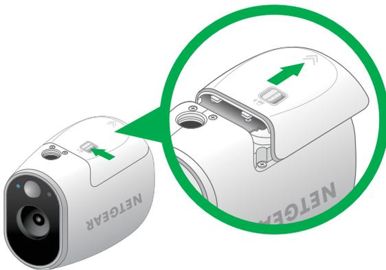
2. Slide the battery door back and lift it to open the battery compartment.
