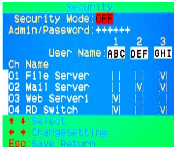
Figure 22: Security setup main window
