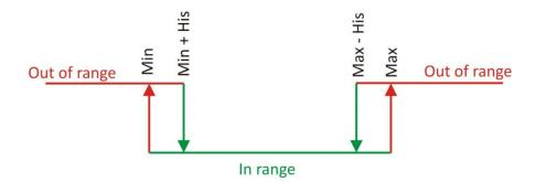
For analog input similar range can be set. It is mandatory that chosen range correspond with the range selection jumper J1 - 0÷5VDC (close) or 0÷100VDC (open).
