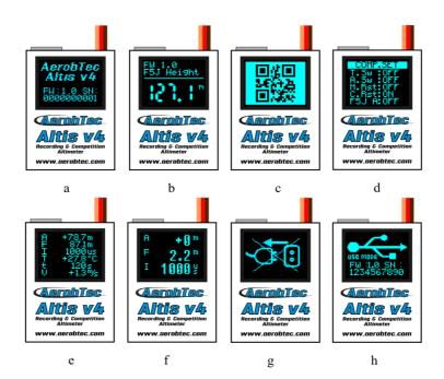
Fig 7: Various screens: a) Initialization screen b) F5J screen c) QR code screen d) Settings screen e)User defined screen with 6 lines e)User defined screen with 3 lines f) Do not disconnect screen g) USB mode screen
