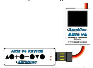
Fig 15: Connection of Altis v4 KeyPad
