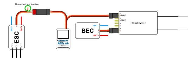
Fig 4: Connection of Altis v4 with BEC
