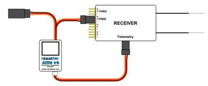
Fig 5: Telemetry connection
