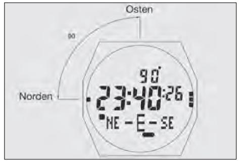
with one bar and the south with three bars. The current direction will be shown at the top of the display in main letters (f. ex. NW-N-NE) The magnetic declination degree is shown on the upper level. All values include: current position, the angle between the local magnetic field (which is the direction the needle of a compass points) and the true north. The declination is positive when the magnetic north is east of true north.
