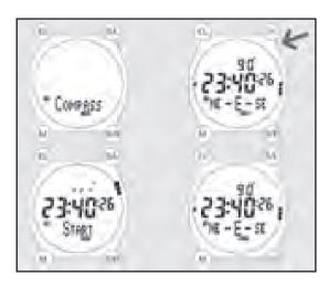
edge of the display, 3 bars indicate "south". After one minute the watch will go into standby mode. To reactivate the compass mode, shortly press the S/L key.
