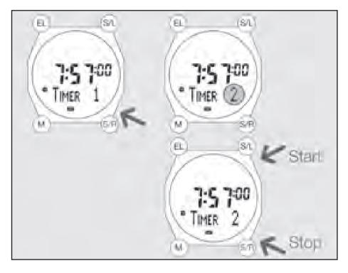
To start the countdown, shortly press the S/L-key. The countdown will go until 0 and the last 5 seconds will be signalled with short beep
