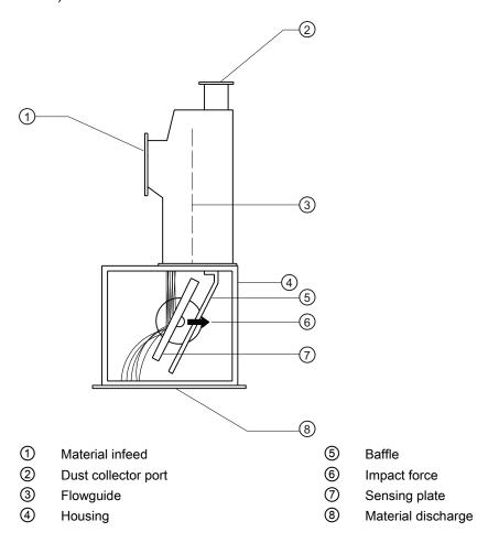
The flowmeter sensing head LVDT output signal is processed by the integrator (ordered separately) to:
