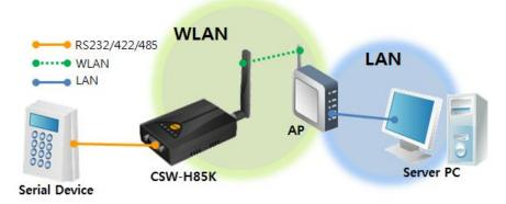
Figure 1-2 1:1 network with a PC through an AP
