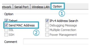
Figure 7-6 setting of Sending MAC Address function
