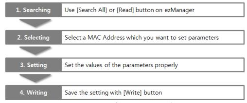
Figure 3-2 configuration via network
