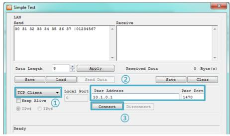
Figure 2-11 settings for TCP connection
