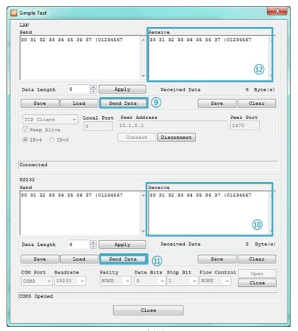
Figure 2-15 successful data transmission
