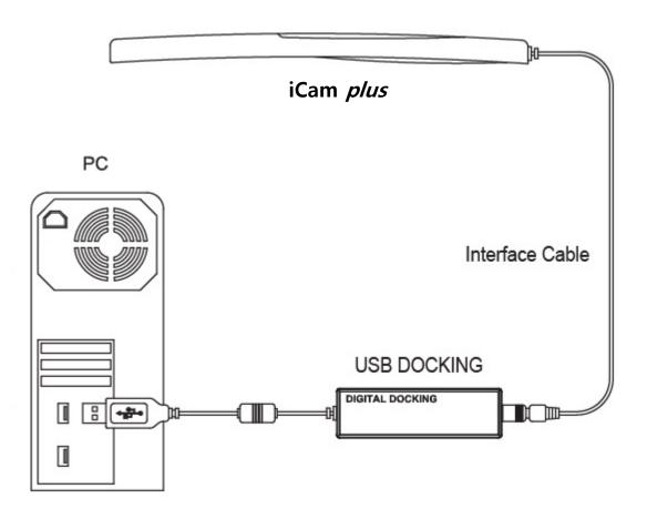
Figure 2.3 Connection diagram of Digital Dock
