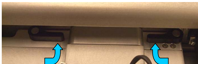
Figure 4.1 Ion source locking knobs.
