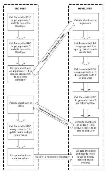
Figure 2: Remote Update Process Using API Calls
