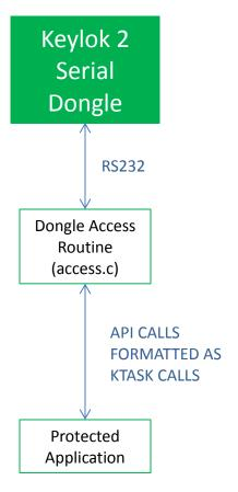
Figure 3: Serial Dongle Access
