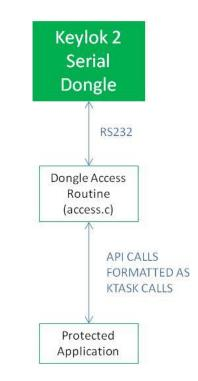
Figure 1: How Dongles Communicate with a Protected Application
