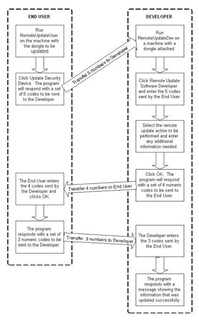
Figure 4: Telephone Remote Update Process
