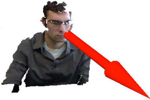
Fig. 1. A point cloud view of a user showing the user's head pose estimate as a vector.
