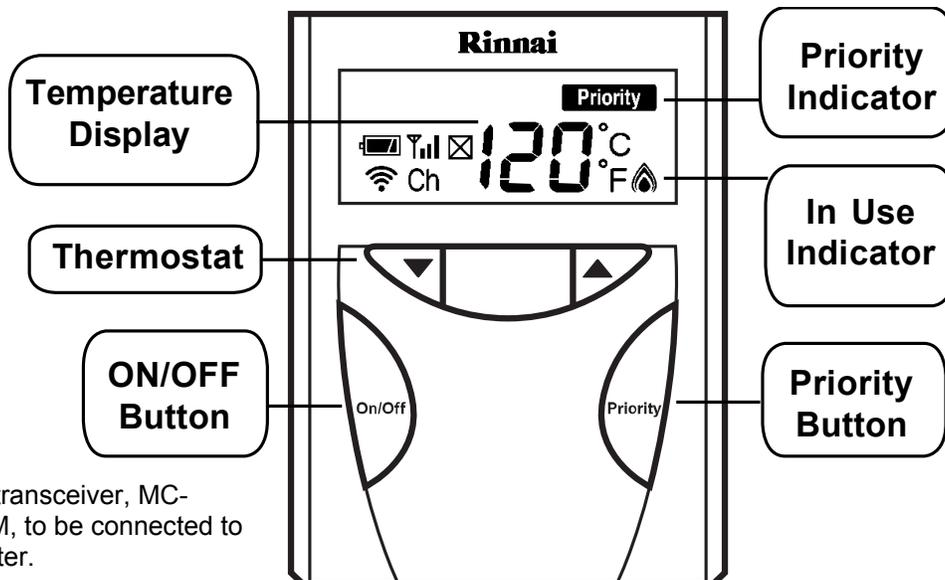
\* Requires the transceiver, MC-502RC-1US-M, to be connected to the water heater.
