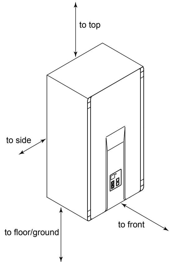
\* 4 inches (102 mm) for enclosed area; 1 inch (26 mm) for unenclosed area.
