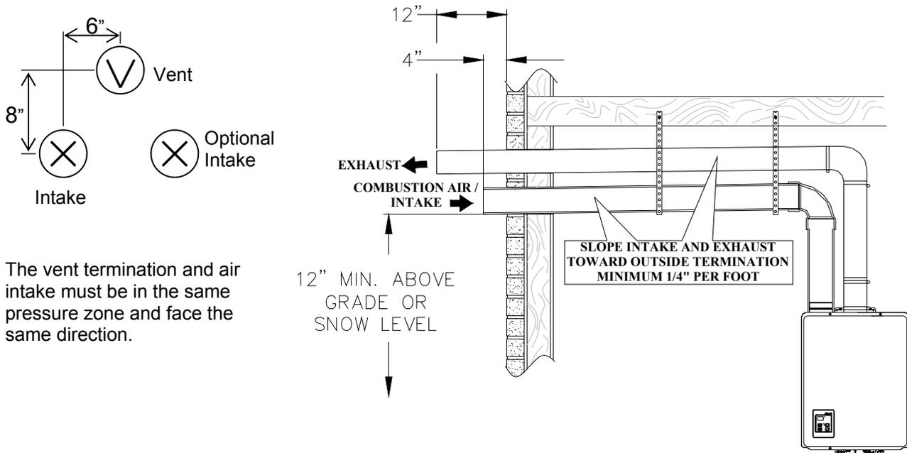
The vent termination and air intake must be in the same pressure zone and face the same direction.
