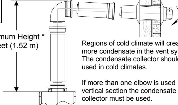
Regions of cold climate will create more condensate in the vent system. The condensate collector should be used in cold climates.
