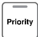
1. Press the "Priority button" on the temperature controller. The green Priority light will glow indicating that this controller is controlling the temperature and that the Rinnai water heater is ready to supply hot water.
