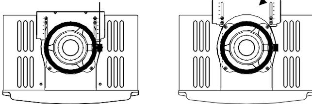
To adjust the condensate collector position or to replace the female vent top with a male vent top:
