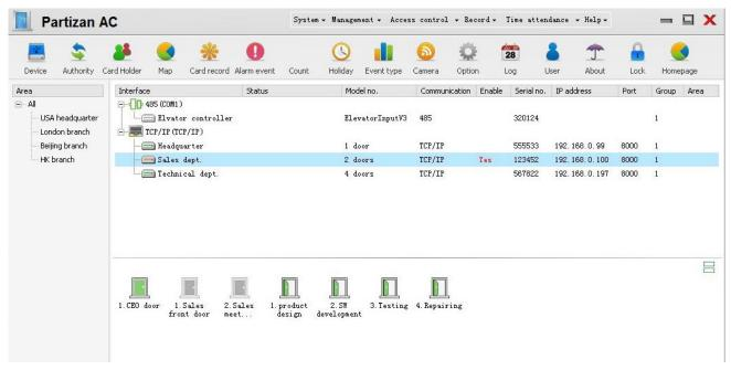
The default interface is the upper interface [access equipment] management interface (you can change the default interface according to the need) after the access control software running, the interface can manage the serial port, controller, door parameter, door operation, area, etc, also can real-time monitoring door state and the event log.
