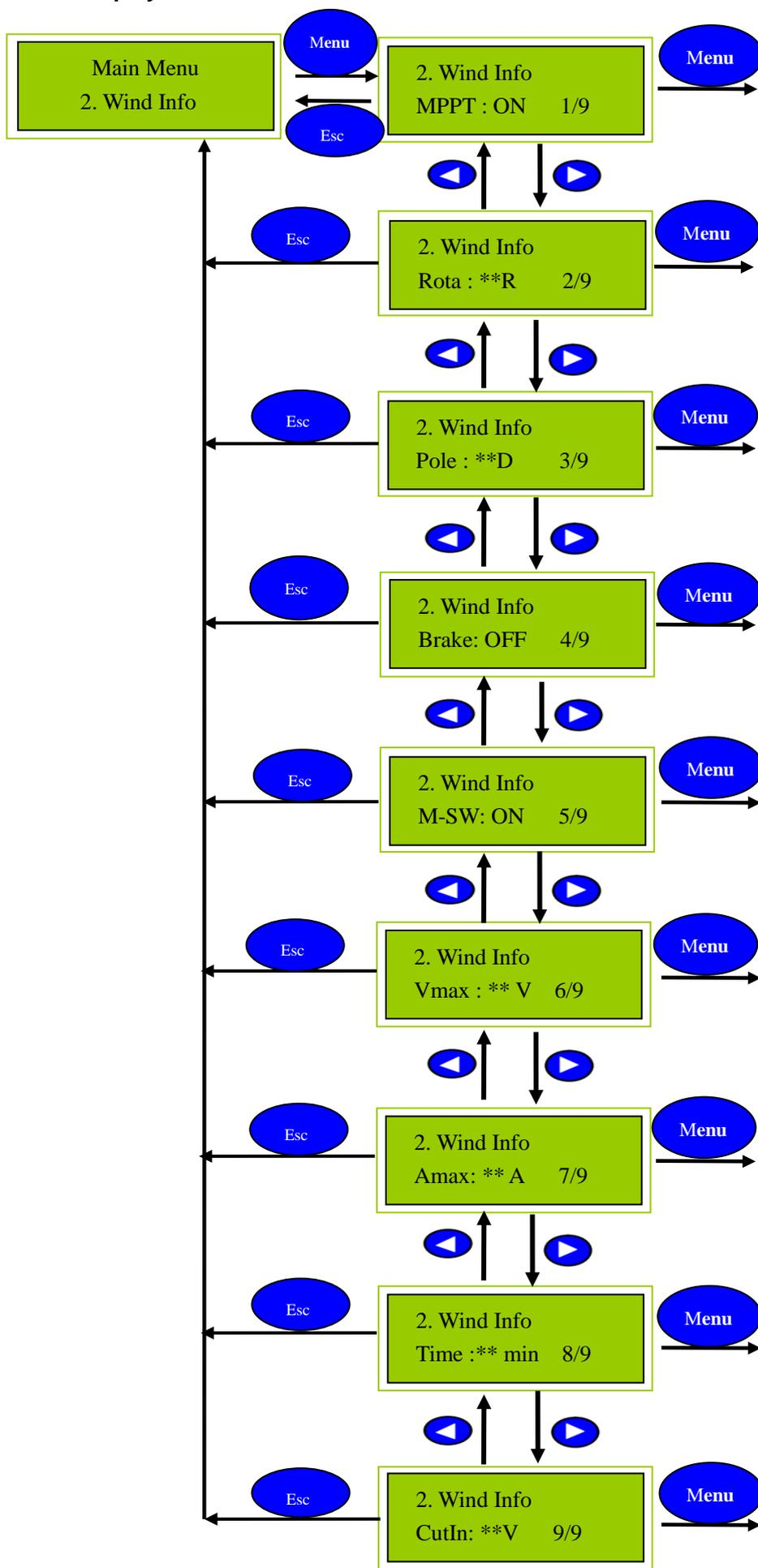
Wind turbine maximum limiting rotate speed numeric flickers. Press and to increase/decrease the value. Press "Menu", saved; Press "Esc", not saved.
