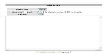
the time the hard drive have to be inactive in order for the LanDrive to enter sleep mode.
