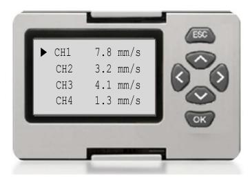
The vibration values coming from the analogical inputs are shown in four lines.
