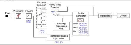
Processing of 4...20 mA analog inputs on Control Card (analog channel ISA00 and ISA01)
