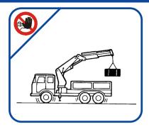
The entire structure of the crane is designed and built to carry the loads shown in the table and with the arms positioned between the horizontal and maximum vertical axes. For this purpose, you must never apply loads to arms with a different configuration (e.g. negative arms). You must also never apply downward pressure with crane arms.
