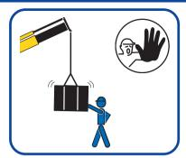
• The workmates of crane operators often have the terrible habit of standing underneath a load that is being moved or to use their hands to accompany the load:
