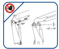
Cranes are only stable when the stabilizers are fully extended - avoid blocking their exit.
