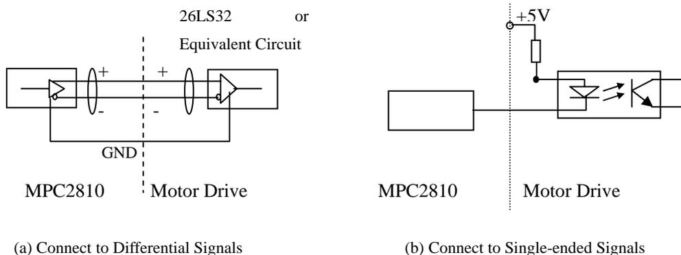
Fig. 3-5 Wiring of Controlling Signals
