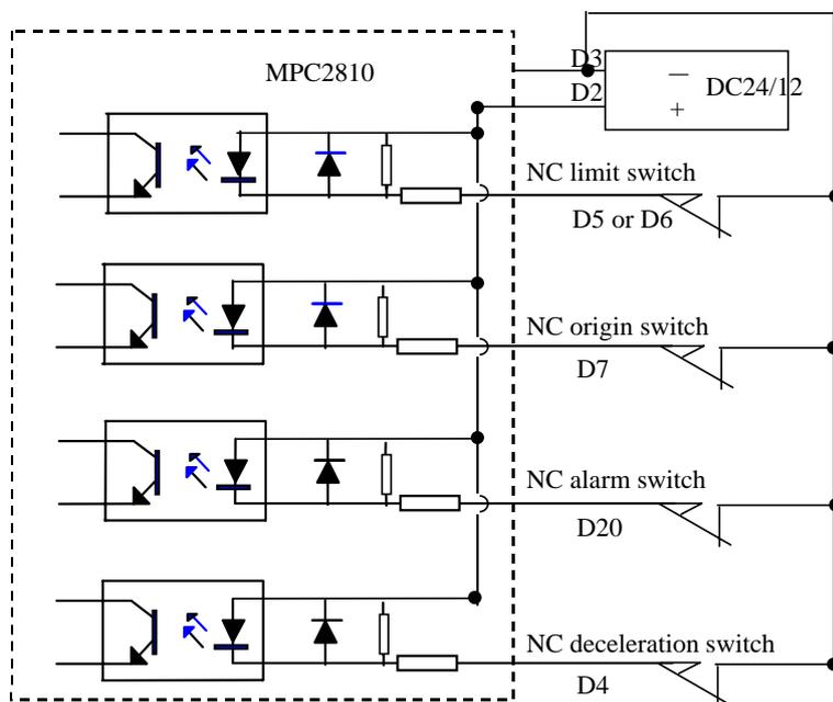
Fig.3-10 Special Inputs Connection Diagram
