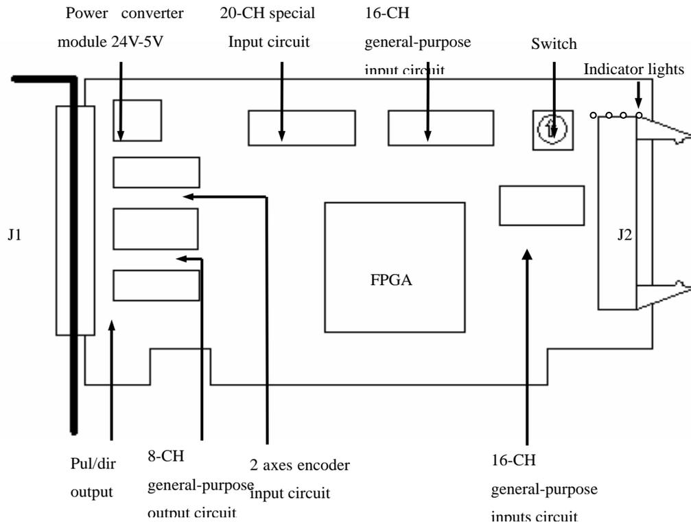
Fig. 2-1 MPC2810 Layout Diagram
