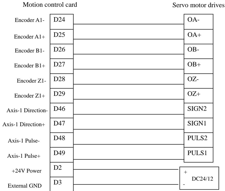
**Note: The encoder feedback pins can be disconnected.**
