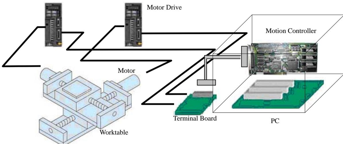
Fig.1-1 Controlling System Applying MPC2810
