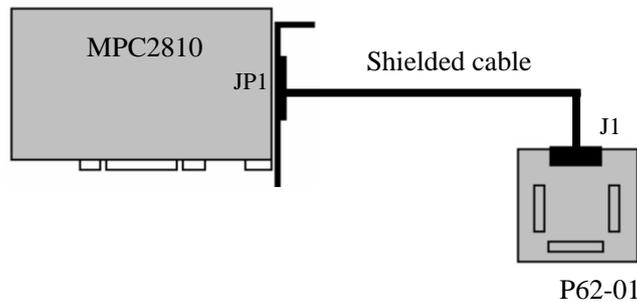
Fig. 3-3 Connect Motion Control Card To Terminal Board
