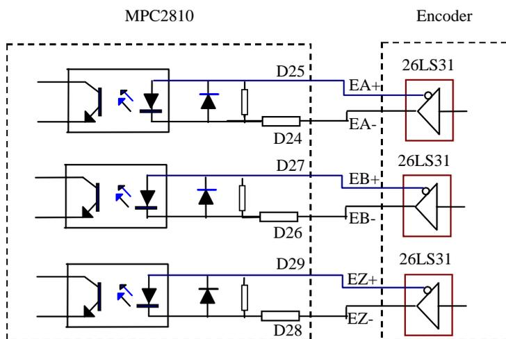
Fig. 3-8 Connection Diagram of Encoder Inputs (Differential-ended)
