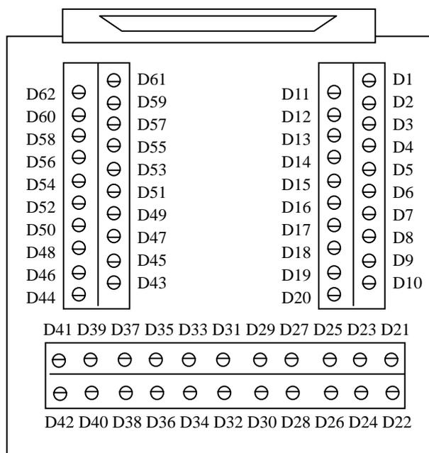
Fig. 3-2 P62-01 Terminal Board Layout Diagram
