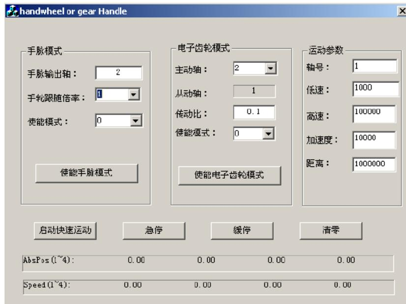
Fig. 2-17 HandwheelorGearHandle window
