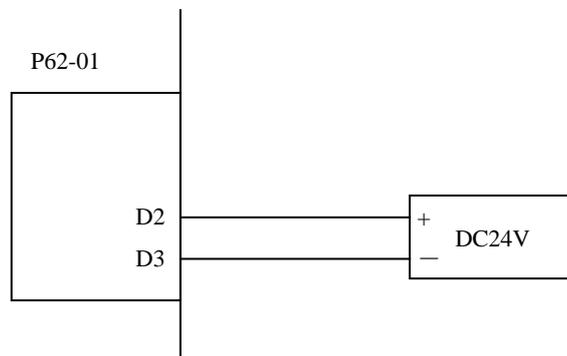
Fig. 3-4 Connect Terminal Board to Power Supply
