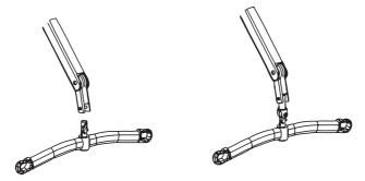
**NOTE** - ENSURE the spreader bar is securely installed before usage.
