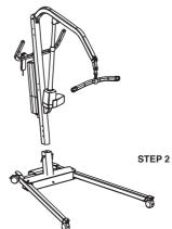
2. Loosen the knob on the mast, lift the mast and boom assembly and fold carefully toward the legs. Use the push handle to assist this motion.
