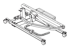
Figure 2 - LIFT IN STORAGE POSITION
