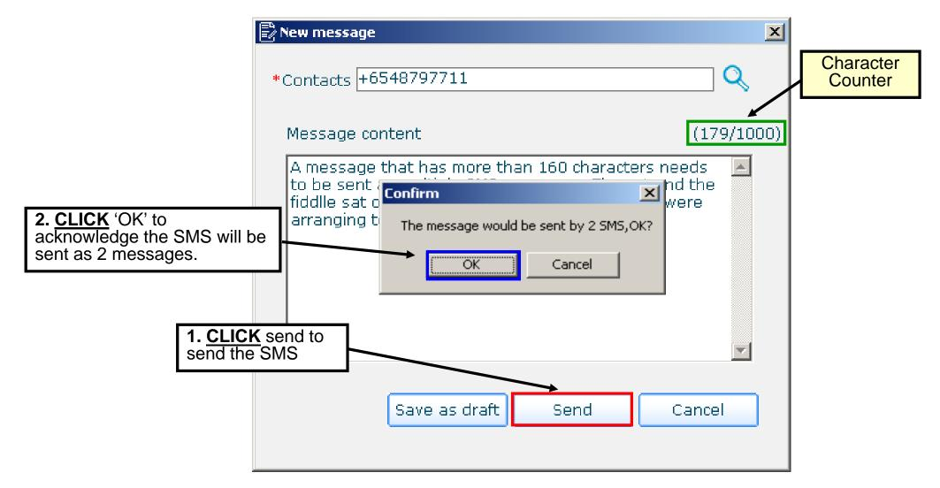
☐ The maximum length of an SMS is 160 characters by default. If this maximum is exceeded the SMS will be sent as 2 SMS.
