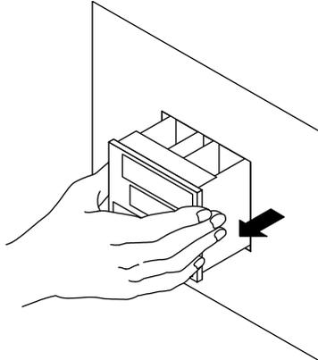
5. The location and number of the relays differ depending on the model code of the UT750. Confirm the location of the control output relay to be replaced before pulling out the relay.
