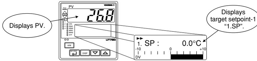
In steps 2 and later, illustrations of the LCD are cited to explain the procedure.
