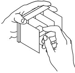
Insert the new relay in the socket. Use the following relay.
