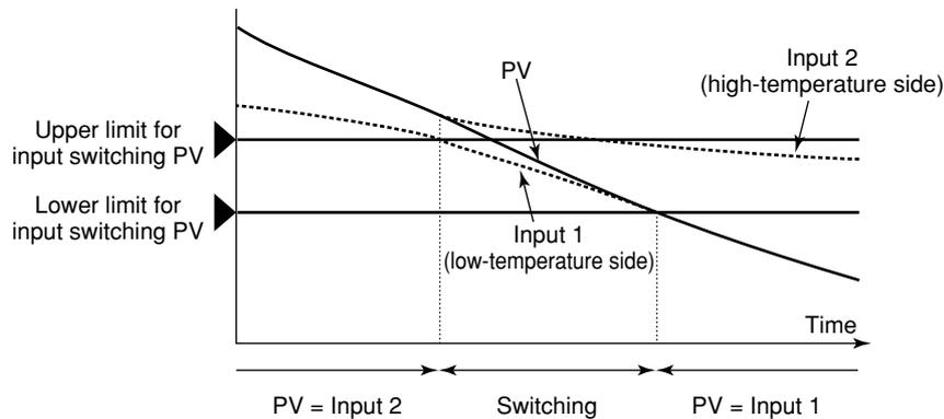
**Switching within Specified PV Range (Falling PV)**
