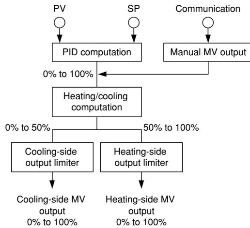
Heating/cooling control provides two methods in which either none of the heating- and cooling-side outputs are presented or both of the heating- and cooling-side outputs are presented, as shown in the following figures.
