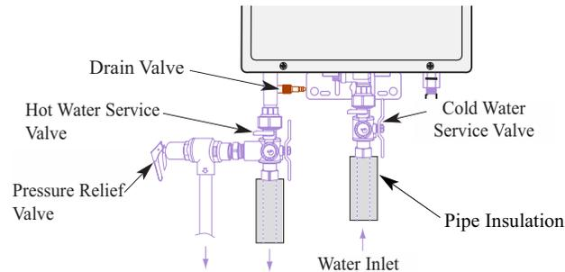
For increased energy efficiency, use pipe insulation. Please install the insulation according to the diagram above, making sure
