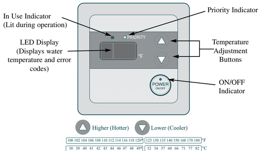
**Notice:** Only heavy duty water heaters can achieve temperatures up to 180°F (82°C).
