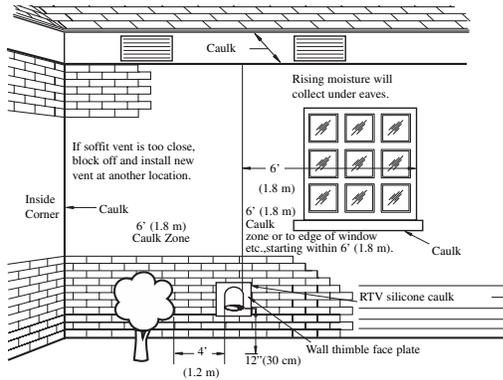
**⚠ WARNING:** Moisture in the flue gas will condense as it leaves the vent terminal. In cold weather this condensate can freeze on the exterior wall, under the eaves and on surrounding objects. Some discoloration on the exterior of the building is to be expected. However, improper location or installation can result in severe damage to the structure or exterior finish of the building.
