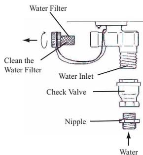
**Notice:** Use only teflon tape on cold and hot water connections and lines.
