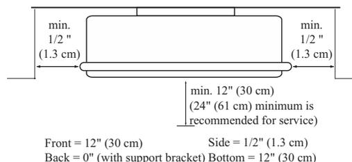
**Top: Do not install this water heater under an overhang less than 36" (91 cm) from its top. The area under the overhang must be open on 3 sides.**
