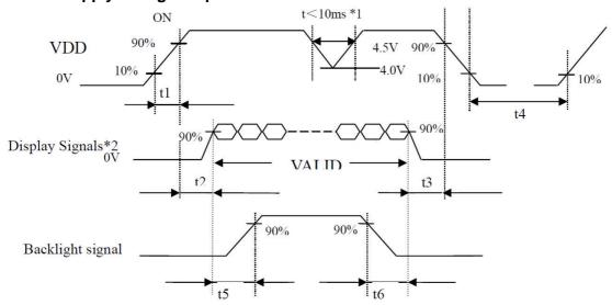
**Timing:** 0.47ms<t1 <10ms; 0.5 ms<t2 <50ms; 0ms<t3 <50ms; t4 >1000ms; t5 >200ms; t6 >200ms; \*1. When VDD is on, but the value is lower than 4.5V, a protection circuit may work, then the module may not display.
